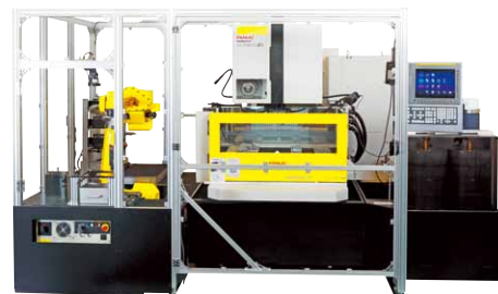
Work-piece exchange cell with Robot
